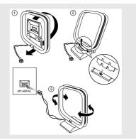
Position the antenna as far as possible from a TV, VCR or other radiation source.
